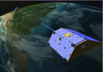
By measuring changes in the distance between the GRACE mission's lead satellite and trailing satellite, scientists can determine changes in the Earth's gravity. (Image courtesy of NASA Jet Propulsion Laboratory)
