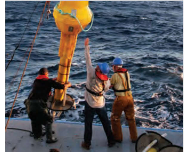
Crew onboard the Thetys research vessel recover Marisonde drifting buoys from the northwestern Mediterranean Sea. The buoys collected sea surface and air measurements for an oceanographic campaign in May 2013. (Courtesy M. Herrmann)
