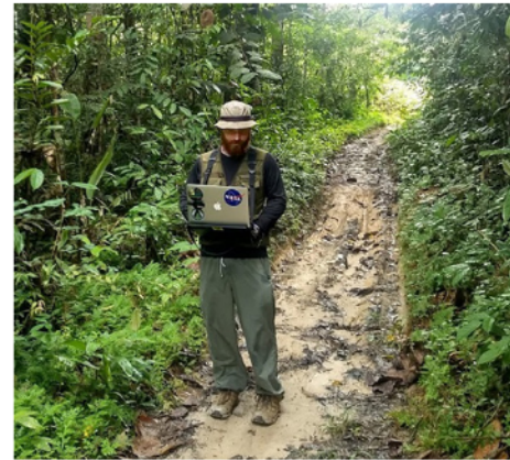
Dr. Bullock looking at historical Landsat data in the Amazon near Iquitos, Peru. Thanks to a Global Positioning System (GPS) hooked up to the computer and a hard drive containing Landsat data, Dr. Bullock is looking at data for the location at which he is standing. These data are helping fine-tune the CODED algorithm for mapping degradation and deforestation across the Amazon Ecoregion. For more information about this research, please see Bullock, E.L., et al. (2020), doi:10.1111/gcb.15029 .
