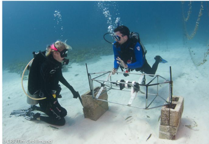
© CRF/Tim Grollmund Dr. Barnes (on right) and a colleague install an optical water quality sensor at a coral nursery in the Florida Keys. Along with satellite-acquired data, Dr. Barnes uses a variety of field-collected data in his research. Image by Tim Grollmund.
